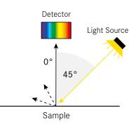
For the blue sample shown beside, a diffuse/8° (also called sphere) geometry instrument will tell you that the sample is the same color on both sides. A 45°/0° (or 0°/45°) geometry instrument will indicate that the halves are different. Which is right? That depends on your need.
