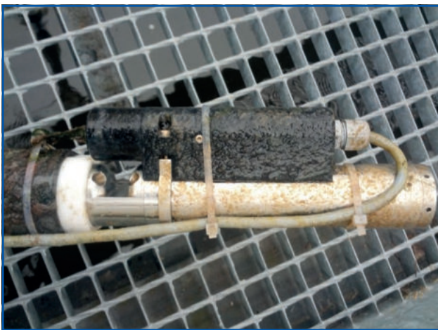
spectro::lyser with efficient automatic cleaning
