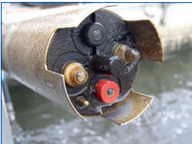
ammo::lyser in waste water effluent
