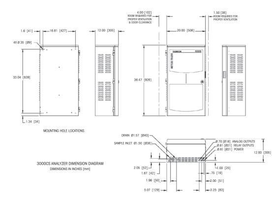
**Note:** Allow 100mm [4in] on left of analyzer for door opening. Allow 38mm [1.5in] on right for ventilation
