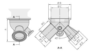
SEFC Sanitary Elbow Flow Cell, reduced inlet (-W1, -W2, -W3)
