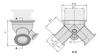
SEFC Sanitary Elbow Flow Cell (-W4, -W5, -W6)
