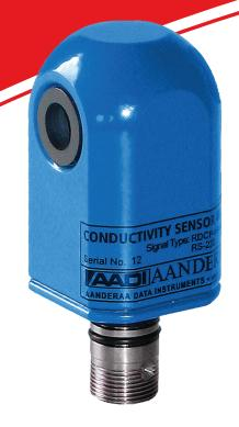
The Conductivity Sensor 4319 is a compact fully integrated sensor for measuring the electrical conductivity of seawater. It is designed to be used with SeaGuard or SmartGuard datalogger using AiCaP CANbus or as stand-alone sensor using RS-232
