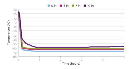
BioT<sup>™</sup> ULT Workstation equilibrates to <-50°C in less than 30 minutes and entire chamber maintains temperature stability for over 15 hours. Temperature measured at 0 inches (blue), 4 inches (red), 7 inches (green), 10 inches (lavender).
