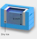
BioT<sup>™</sup> ULT Transporter provides a stable ultra-low temperature (< -70°C to -50°C) work zone 8.0 inches (20.3 cm) deep. Up to 8 standard 2-inch cryostorage boxes will remain safely below -50°C for over 8 hours with the lid open and over 24 hours with the lid closed with one charge of dry ice.
