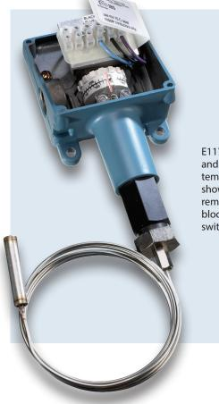
E117 bulb and capillary temperature switch shown with cover removed. Terminal block with SPDT switch output.
