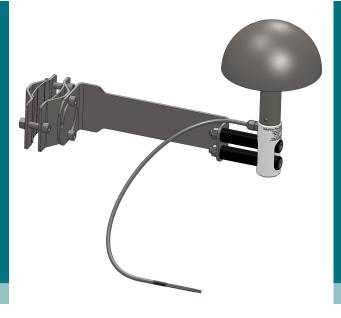
The RHD is a low-cost, high precision, ultra-robust rain gauge. It features very low- power consumption, is maintenance- free and has a completely sealed acoustic sensor with no moving parts. The sensing device is a polished stainless steel hemisphere supported by a strong stainless steel arm. It detects changes of the acoustic pressure that are induced by the impact of raindrops or hailstones. The RHD also includes a distrometer that return the drop size distribution.
