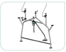
Pic: RHD on a sensor rack of a wind turbine
