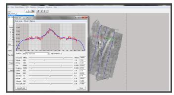
Generate mosaics from side scan data, multibeam backscatter or multibeam snippets in GEOCODER™. Licensed from UNH-CCOM, it's a standard feature in HYPACK®.
