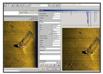
HYPACK<sup>®</sup> supports collection, targeting and mosaicking for both analog and digital side scans. It's a standard feature!
