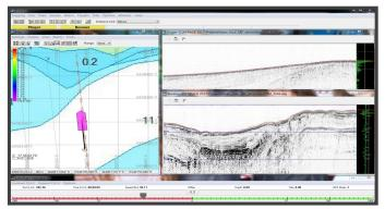
HYPACK<sup>®</sup> supports both analog and digital sub-bottom systems. It saves your data to industry standard SEG-Y. It's a standard feature in HYPACK<sup>®</sup>.
