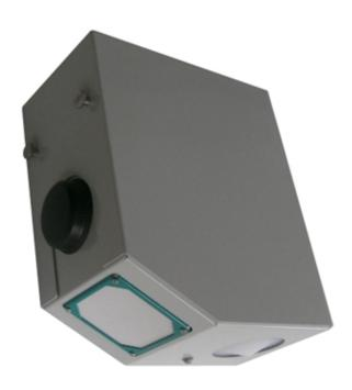
The RQ-30 ADMS is an all-in-one discharge measurement system, suitable for spot-measurements, temporary applications or stationary long-term installations. It contains the contactfree flow velocity and water level sensors of the RQ-30 and applies the same algorithms to compute the water discharge.
