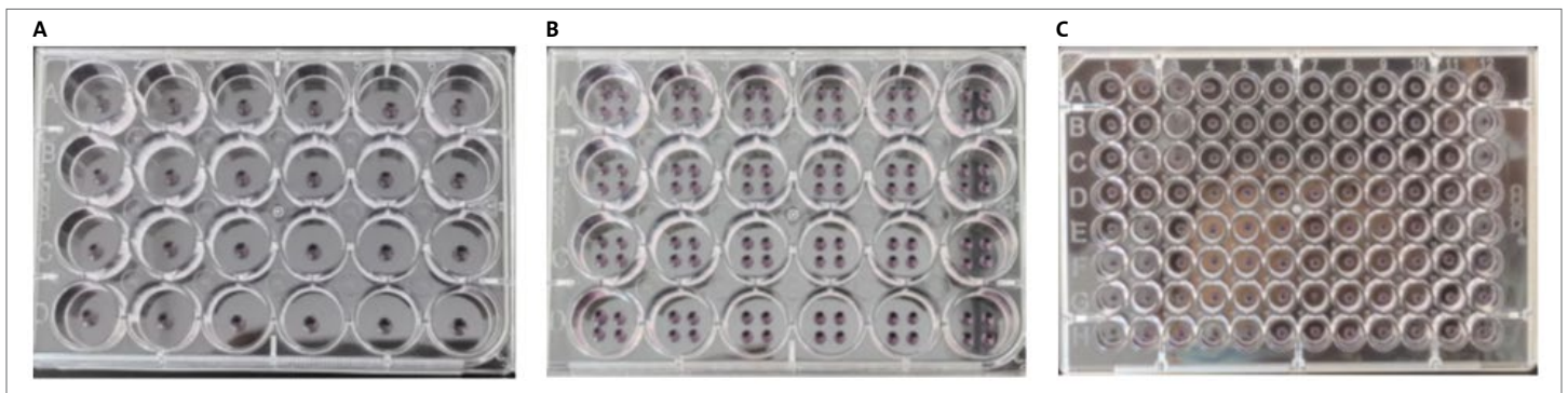
Figure 2. Uniform domes of 9 mg/mL Corning Matrigel matrix formed in each well.
