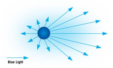
**LIF**: Molecule is excited to a higher energy level laser light source, then releases that energy by emitting fluorescence
