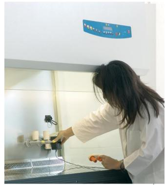
**Prefilters removal**: prefilters can be removed directly from the working chamber
