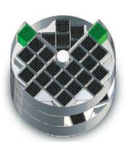
The upper level provides a convenient workspace where canisters can be parked (shown in green) and samples inspected at -190°C.
